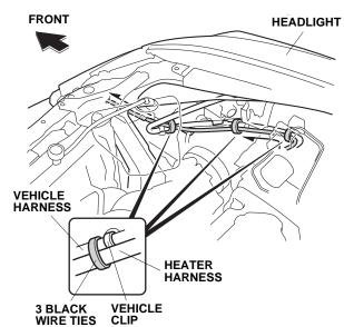
23. Route the heater harness as shown, and secure the wire tie with clip (point G) to the vehicle frame.
