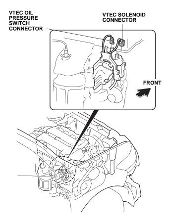
14. Release the harness holder from the VTEC bracket (two hooks).
