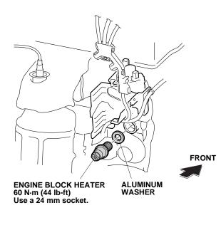
17. Plug the connector end of the heater harness into the engine block heater. Route the heater harness as shown, and secure the two wire ties with clips (points A and B) to the vehicle bracket.
