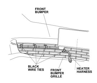
26. Attach the protective cap to the front bumper grille, and plug the connector on the heater harness into the protective cap.
